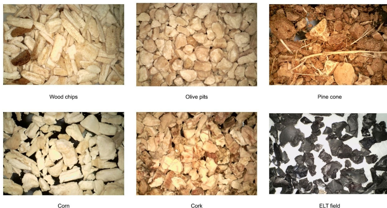
Fig. 1 Visual comparison of six alternative infill materials for sports surfaces: a Wood chips, b Olive pits, c Pine cone, d Corn, e Cork, and f ELT field. Images are shown at a comparable scale; granule sizes range approximately from 0.3 to 3.0 mm depending on the material.
