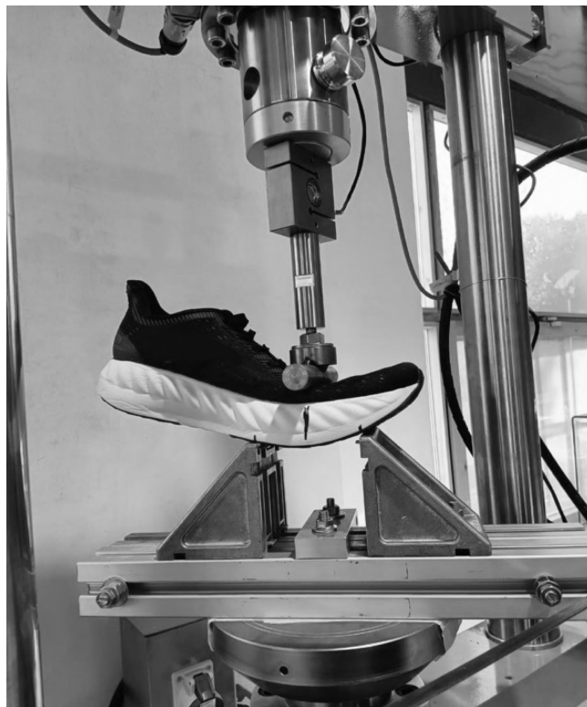
FIGURE 1 Setup of mechanical stiffness test on running shoes.
