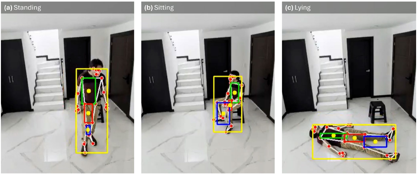
FIGURE 7 | Examples of bounding boxes for the three postures studied ( Standing , Sitting , and Lying ) in real-world images.
