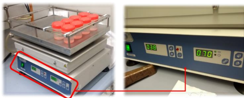
Figure 48. Orbital mixer and shaker with the drug release vessels operating at 70 rpm and heating at 37 °C.
