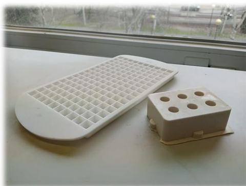
Figure S26. Silicon molds used for the synthesis of the hydrogels.
