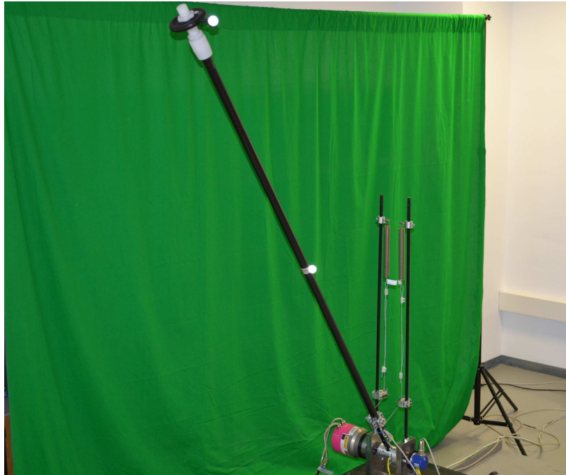
Fig. 7.3 Experimental setup: photograph of the single link flexible robot with the passive gravity compensation system.
