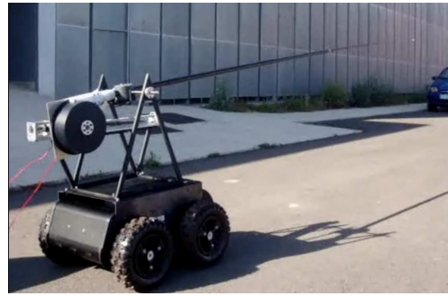
(b) Manipulator B: single-link flexible manipulator with a rotary and a prismatic joint.
