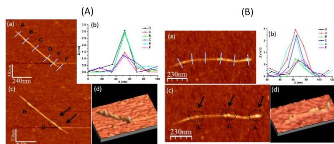
**Fig. 3** (a) Topography AFM images of *f*-SWCNT **3** (panel A) and *f*-SWCNT **4** (panel B) on a SiO<sub>2</sub> surface; the Z-profiles indicated with lines A–F are shown in graph (b); (c) AFM images highlighting the functionalized zones; (d) 3-dimensional images of hybrids **3** and **4**.
