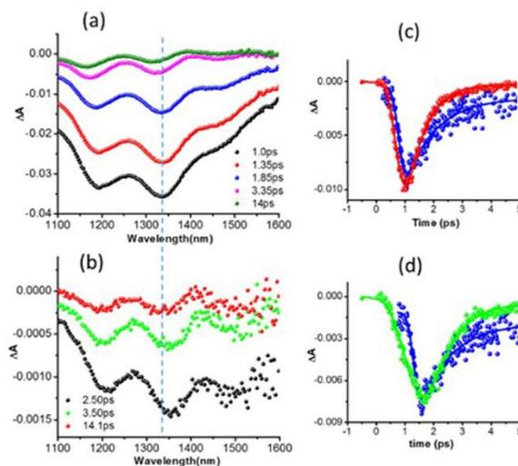
**Fig. 5** Femtosecond transient absorption spectra of (a) pristine SWCNT (HiPCo) and (b) *f*-SWCNT **3** in DMF at the excitation wavelength of 400 nm (100 fs pulse width) at the indicated delay times. (c) Time profile of the 1335 nm peak of pristine SWCNT (blue) and 1353 nm peak of *f*-SWCNT **3** (red). (d) Time profile of the 1335 nm peak of pristine SWCNT (blue) and 1327 nm peak of *f*-SWCNT **4** (green).
