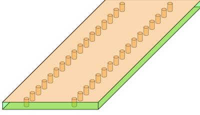
Fig. 1. SIW geometry.
