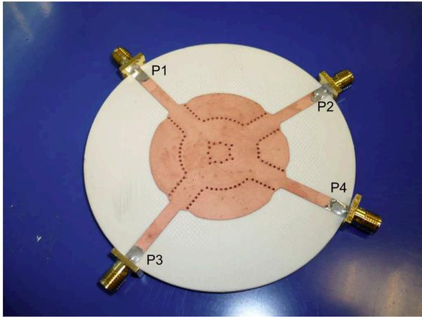
Fig. 8. Fabricated prototype of the hybrid ring of Fig. 4(b) and taper dimensions.
