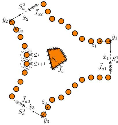
Fig. 2. Arbitrary SIW-based device.
