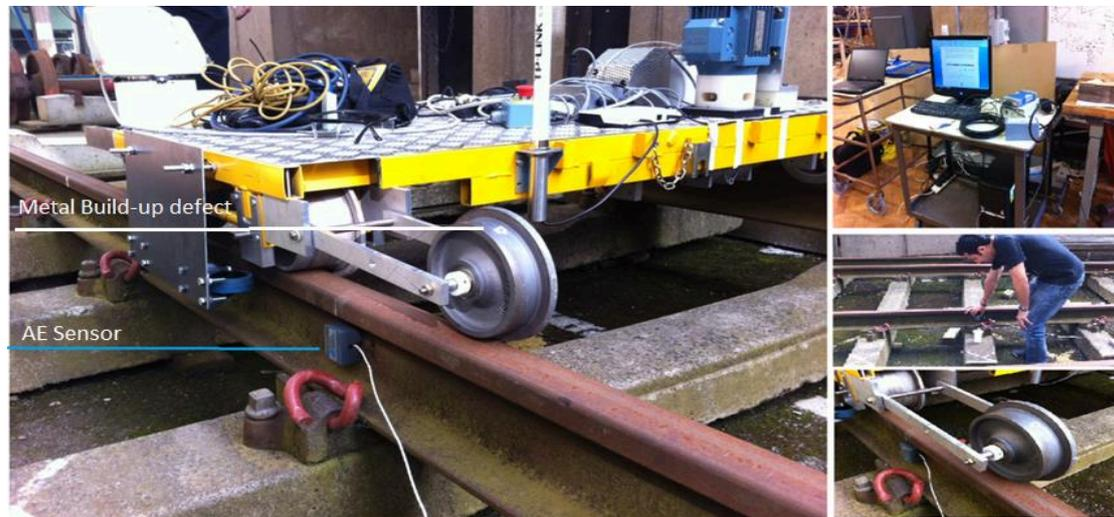
Figure 3: Experimental setup for trolley tests.
